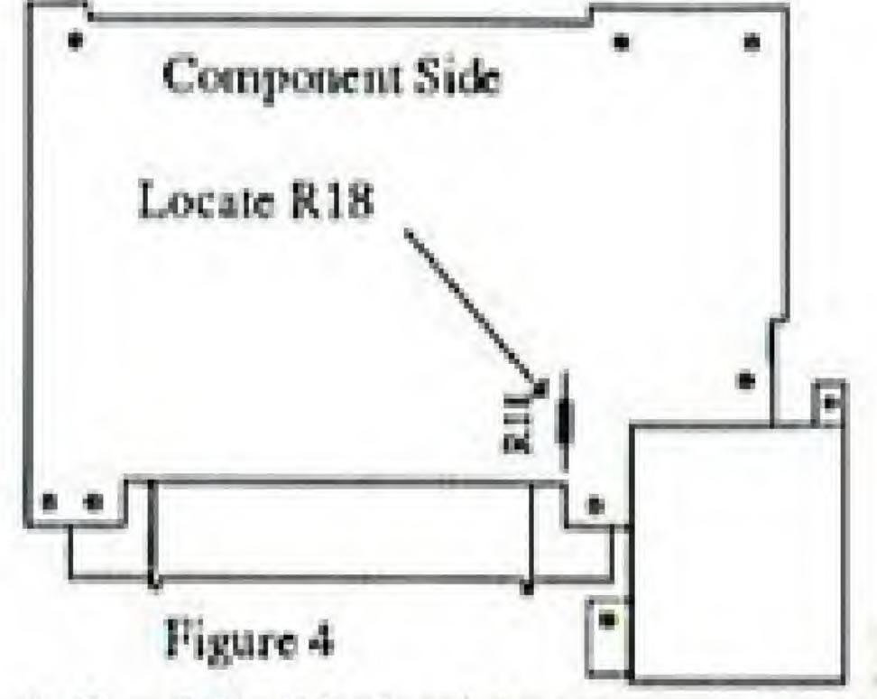
4. Carefully lift circuit board out of bottom and with all wires still attached turn board over. Be sure board is a Rev 11. This will be verified by the presence of R18 as indicated in Figure 4. If R18 is not present do not proceed! Call 1-800-HOT-4-AVE for assastance.
